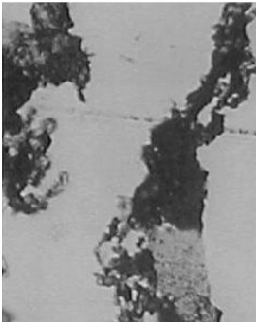
Fig. 7: Particles of ultimate wear, they have potted on the surface caused by repeated passage of zone of rolling contact, they are produced at the end of fatigue wear. Magnification 500 x.
